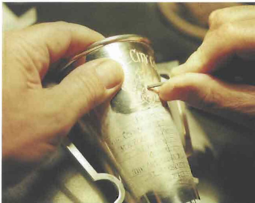
Two stages of engraving of the 2003 Liverpool Cup with the coat of arms and the race details. The sterling silver cup will then be 24ct gold plated
